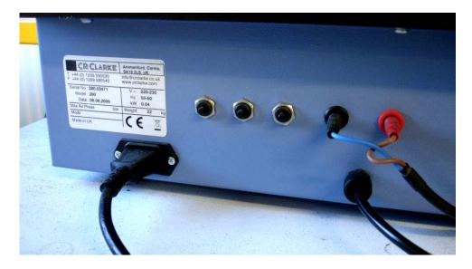
8). Plug the machine into a suitable electrical supply, the power neon will illuminate (green).
