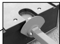
3). Hook the cutting wire over the adjustable brass terminal. The terminal has been preset during testing so that it makes a 90° angle with the depth of the work table.
