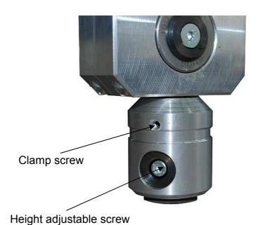
In the clockwise turn sink = Lift machine Turn against clockwise = Sink machine
