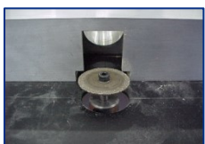
Dust Extraction Fence
