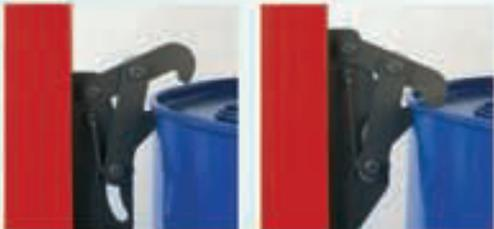
Automatic clamp. Just position the clamp under the tight head of the drum. Both clamping and release are made automatically.
